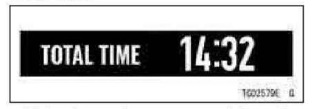
This shows the amount of time that has elapsed while the ignition switch is turned on.
