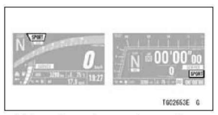
This motorcycle can change its performance characteristics with the press of a button only. This system has three different preset modes and they integrally control the engine.
