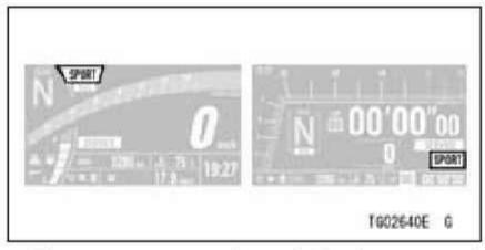
The current setting of the integrated riding mode is shown. Refer to the Integrated Riding Modes section in the HOW TO RIDE THE MOTORCYCLE chapter.
