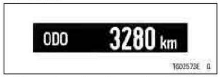
The odometer shows the total distance. This meter cannot be reset.
