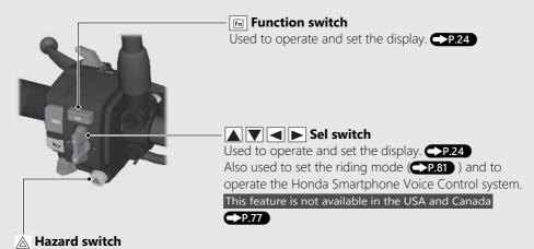
Switchable when the ignition switch is the ON position. You can turn it off regardless of ignition switch position.
