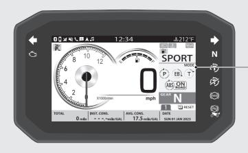
Do not operate the display functions for a long time with the engine stopped. It may result in a low (or dead) battery.
