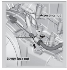
If proper adjustment cannot be obtained or the clutch does not work correctly, see your dealer.
