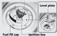
Do not fill with fuel above the level plate.
