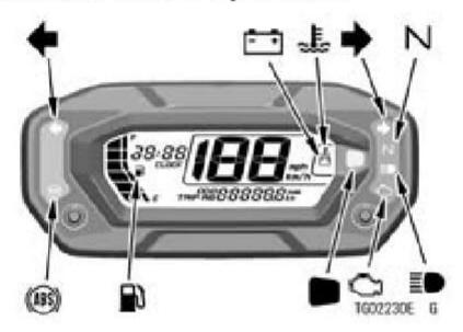
When the ignition switch is turned on, all indicators go on/off as shown in the table. If any indicator does not operate as shown, have it checked by an authorized Kawasaki dealer.
