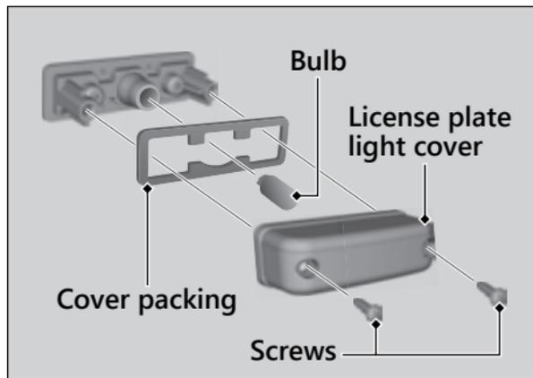
4. Install a new bulb and the parts in the reverse order of removal.
