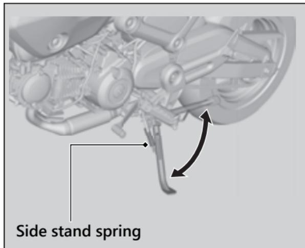
1. Check that the side stand operates smoothly. If the side stand is stiff or squeaky, clean the pivot area and lubricate the pivot bolt with clean grease.
