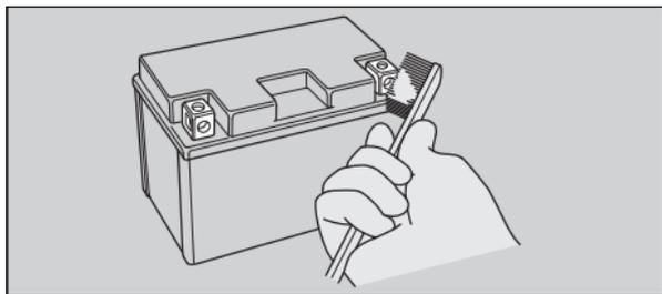
4. After cleaning, reinstall the battery.
