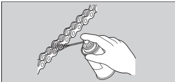
Never use gasoline or low flash point solvents for cleaning the drive chain.
