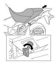
To remove the seat, insert the ignition key into the lock and turn it clockwise. Raise the rear end of the seat and slide it backward.
