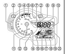
The malfunction indicator light ⑥, freeze indicator light ⑫, engine coolant temperature indicator light/oil pressure indicator light ④, ABS indicator light ⑥, traction control indicator light ⑤, LCD's and tachometer needle work as follows to confirm their function when the ignition switch is turned to the "ON" position.
