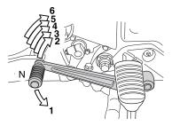
This motorcycle has a 6-speed transmission which operates as shown. To shift properly, squeeze the clutch lever and close the throttle at the same time you operate the gearshift lever. Lift the gearshift lever to upshift and depress the lever to downshift. Neutral is located between 1st and 2nd gear. When neutral is desired, depress or lift the lever halfway between 1st and 2nd gear.
