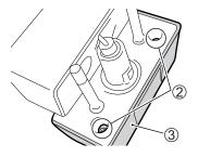
Remove the screws ② and take off the cover with the lens ③.
