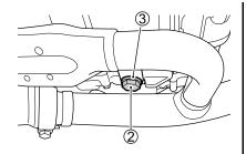
3. Remove the drain plug ② and gasket ③ from the bottom of the engine and drain the engine oil into a drain pan.
