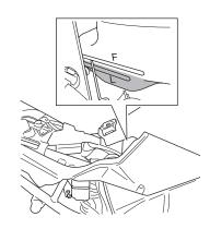
Remove the seat to check the coolant level. The engine coolant solution should be between the "F" (FULL) and the "L" (LOW) level lines on the engine coolant reservoir. If the level is lower than the "L" level line, bring it up to the "F" level by adding specified engine coolant.
