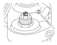
To set the rebound damping force adjuster to the standard position, turn the adjuster clockwise until it stops and then turn it counterclockwise 8 clicks.
