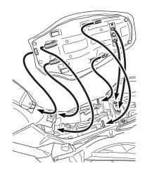
To reinstall the seat, slide the seat hooks into the seat hook retainers and push down firmly until the seat snaps into the locked position.
