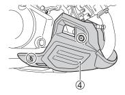
4. Remove the right and left bolts and remove the under cowlings 4.
