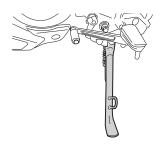
An interlock system is provided to cut off the ignition circuit when the side stand is down and the transmission is in any gear other than neutral.
