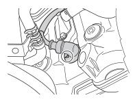
NOTE: When installing the spark plug caps, point the arrow marks on the spark plug caps to the exhaust side.
