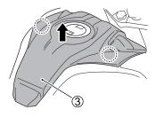
6. Unhook the hooks and remove the front tank cover ③. Covers have hooks at the circled places.
