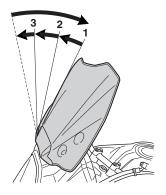
NOTE: After adjusting the windshield angle, check that the locks are fixed in the same positions at both right and left sides.
