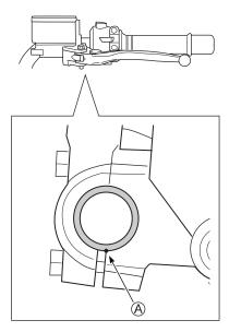
Align the dot mark on the handle-bar with the mating surface of the lever holder  $\widehat{\mathbb{A}}$ .
