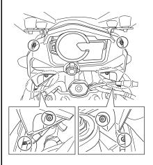
Remove the bolts and fasteners.
