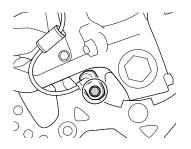
2. Remove the front wheel speed sensor by removing the mounting bolt.
