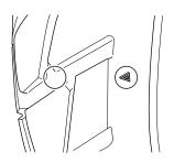
NOTE: The "\(\triangle \)" mark indicates the place where the wear bars are molded into the tire. When the wear bars contact the road, it indicates that the tire wear limit has been reached.
