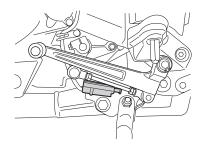
Check the side stand/ignition interlock system for proper operation as follows:
