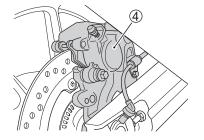
8. Remove the rear brake caliper assembly 4.
