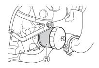
5. Turn the oil filter ⑤ counter-clockwise with a Suzuki "cap type" oil filter wrench or a "strap type" filter wrench of the proper size.
