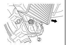
Remove the radiator mounting bolt ② and slide the radiator forward.
