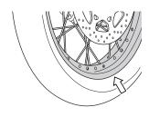
Check to see if there is any damage like crack, distortion or bend in the wheel rim.
