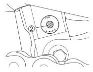
The rebound damping force adjuster ② is located at the bottom of the rear suspension damper unit. To adjust the damping force, set the adjuster to the standard setting first and then adjust it to the desired position.
