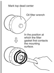
Tighten the filter 2 turns or to specified torque.
