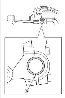
Align the dot mark on the handle-bar with the mating surface of the lever holder  $\widehat{\mathbb{A}}$ .
