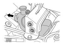
Remove the reservoir tank mounting bolts and move the reservoir tank forward.
