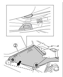
Remove the bolts. Pull the right and left side frame covers 2.
