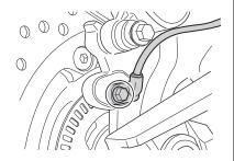
2. Remove the rear wheel speed sensor by removing the mounting bolt.
