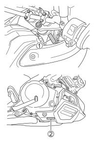
The frame number ① is stamped on the steering head as shown in the illustration. The engine serial number ② is stamped on the crankcase assembly.
