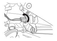
1. Turn the socket ① counter-clockwise and remove it.
