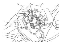
The main fuse is located under the seat. One 30A spare fuse is located in the starter relay box.
