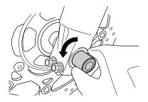
9. Turn the axle shaft counterclockwise and draw it out.
