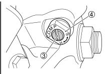
To set the compression damping force adjuster to the standard position, turn the adjuster clockwise until it stops and then turn it counterclockwise 8 clicks.
