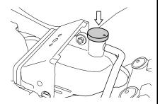
Remove the filler cap and add specified engine coolant through the filler hole until it reaches the "F" line. Refer to the FUEL, ENGINE OIL AND COOLANT RECOMMENDA-TIONS section.
