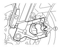
3. Remove both brake calipers from the front forks by removing two mounting bolts ① on each of the calipers.
