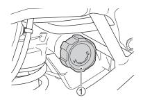
To adjust the rear suspension spring pre-load, turn the adjuster ①.
