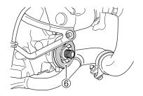
6. Wipe off the mounting surface 6 on the engine where the new filter will be seated with a clean rag.
