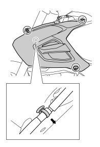
7. Remove the right and left fuel tank side covers bolts. Remove the wiring harness clamp.
