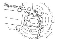
7. With the wheel moved forward, remove the chain from the sprocket.
