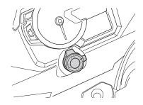
The DL1000A/XA has an output terminal for attaching 12V electrical accessories. Total electrical accessory wattage should be less than 36W. Check electrical accessory voltage and wattage before attaching accessories to the output terminal.
