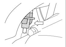
To adjust the brake light switch, hold the switch body and turn the adjuster so that the brake light will come on just before a pressure rise is felt when the brake pedal is depressed.
