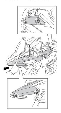
3. Remove the right and left bolts. Unhook the hooks and remove the right and left side covers ①.
