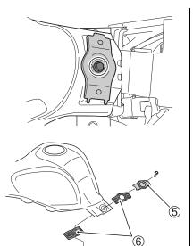
9. Remove the bolt. Remove the prop ⑤ and two cushions ⑥.
