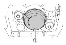
1. Turn the cap ① counterclockwise and remove it.
