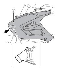
8. Slide the right and left fuel tank side covers ④ forward to slip off the hook. Remove the right and left fuel tank side covers ④.
