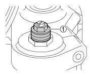
To change the spring pre-load, turn the adjuster ① clockwise or counterclockwise. Turning the adjuster clockwise will increase the spring pre-load. Turning the adjuster counterclockwise will decrease the spring pre-load.
