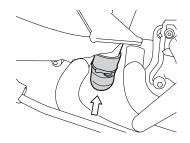
Remove the plug and drain water and oil at the periodic maintenance interval. The air cleaner drain plug is located beneath the air cleaner box.
