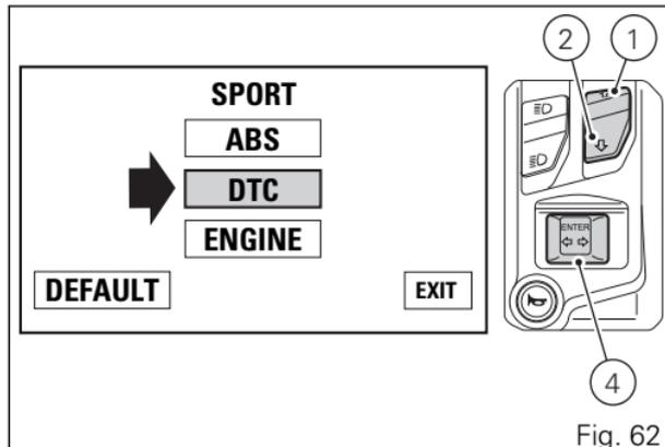
When entering the function, the currently set DTC level or status is indicated on the left (e.g.: DTC 3). Customisation options are indicated in the middle: levels 1 to 8 and status OFF. Select the parameter to be customised (DTC), by pressing button (1) or (2). Once the desired parameter is highlighted, press CONFIRM MENU button (4). To save the new setting, hold button (4) for two seconds while the message MEMORY is highlighted in orange.
