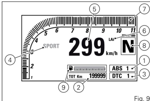
From the main screen, with CORE layout, press button (1) on LH switch to view Menu 1 information.
