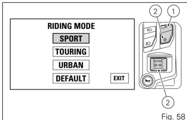
Press buttons (1) and (2) to highlight the customisable parameters one by one: in particular, use button (1) to highlight the following item and button (2) to highlight the previous item.
