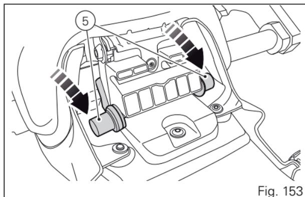
Fit the seat with its cover on the motorcycle. Now the seat is in a lowered position.
