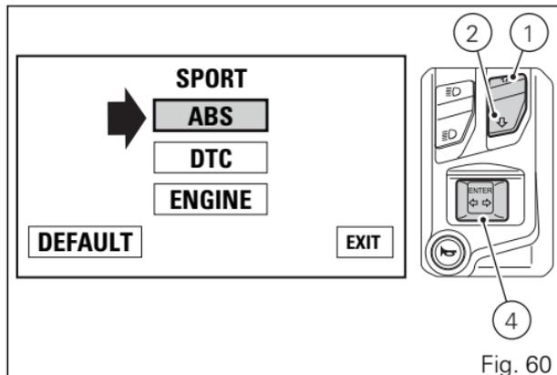
When entering the function, the currently set ABS level or status is indicated on the left (e.g.: ABS 1). Customisation options are indicated in the middle: levels 1 to 3.
