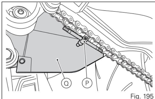
Slide out pin (P) and fasten battery mount cover (16) using screws (15); tighten them to  $5 \text{ Nm} \pm 10\%$ . Fit the positive cable (13) and ABS positive cable (14) on battery positive pole and fasten it by tightening screw (12) to  $10 \text{ Nm} \pm 10\%$ .
