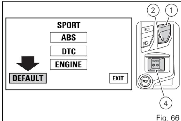
It will take 3 seconds to restore parameters, during which PLEASE WAIT ... will appear on the display. Once procedure is completed, DEFAULT OK will appear for two seconds to confirm that default parameters have been restored. The display then automatically goes back to Riding mode customisation menu first page, with EXIT option highlighted. To quit the menu and go back to Setting Menu main page, select EXIT and press button (4).
