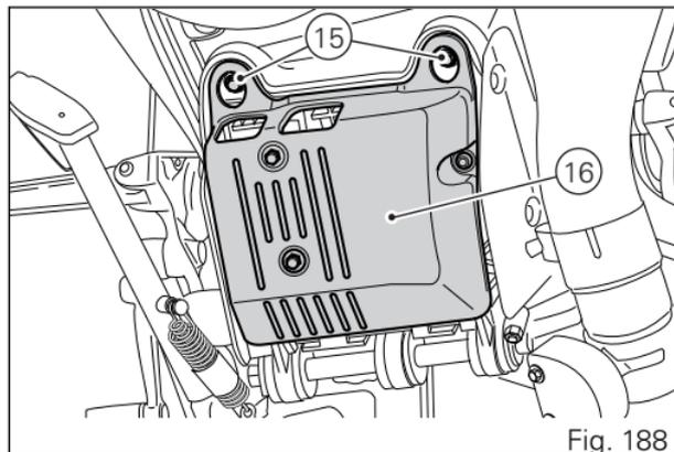
Turn battery mount cover (16) down and remove service pin (P) while supporting the battery (17) with your hand.
