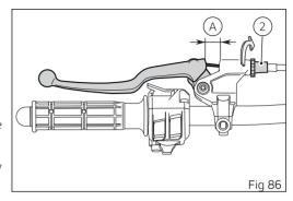
Adjuster (2), located on the lever, allows a maximum adjustment (Q) of 11 mm (0.4 in), whereas the standard adjustment (starting one) is of 5 mm (0.2 in). If working on such adjuster proves insufficient, work on the secondary adjuster (3).
