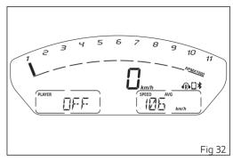
On instrument panel, Menu 1 PLAYER option and the active track name (C) are displayed. together with the Player menu. If the Player is turned on, button (1), button (2) and button (4) can only be used to control the PLAYER.
