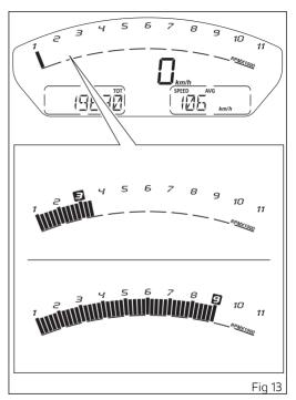
When the thresholds before the rpm limiter are reached, the corresponding warning lights will turn on.
