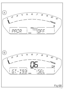
The list of devices found within the range during the Pairing stage does not include already paired devices, even if their Bluetooth connection is ON. The name of the device is scrolled on the display. To pass from one device to the other, press buttons (1) and (2).
