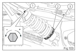
spring preload: ± 5 mm (0.2 in) with respect to the nominal position, from 10 ÷ 20 mm (0.4 ÷ 0.8 in) from fully closed.
