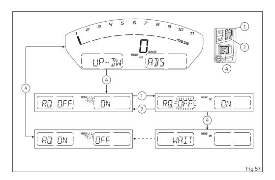
If the ABS is in fault, "ERR" is displayed in Menu 2 when entering the function and Menu 1 will indicate "NO RQ.", since no selection is actually possible. "EXIT" box is flashing. Press button (4) to quit the function.
