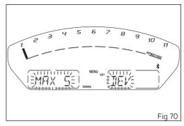
When device is selected, the user must indicate the type of connected using buttons (1), (2) and then button (4) to confirm. Types of devices can be:
