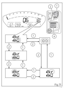
To pair a Smartphone, the pairing procedure with the Bluetooth control unit requires user to enter a code (0000), which is only necessary the first time the device is paired with the Bluetooth control unit. In this case, the Instrument panel displays the PIN to be entered: "0000" in Menu 1, "PIN" in Menu 2 and the Smartphone icon flashing.
