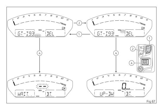
At the end of the pairing, the number of the detected devices is displayed.
