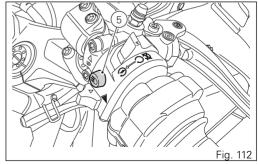
High/low beam switching off during vehicle start (version without DRL light).
