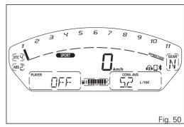
On instrument panel, Menu 1 PLAYER option and the active track name (C) are displayed. together with the Player menu. If the Player is turned on, button (1), button (2) and button (4) can only be used to control the PLAYER.
