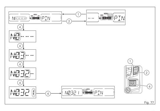
When you press button (4) to confirm the fourth and last digit, the instrument panel highlights the message "MEM" and the relevant box.
