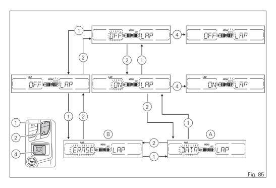
The LAPs previously stored using the "LAP Recording" function in the Menu can be viewed on the display.
