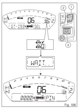
If you wish to connect a Bluetooth Navigator, the connection procedure shall be completed on the navigator, by selecting the connection with the motorcycle Bluetooth control unit. In this case, during the pairing procedure, the Navigator icon will flash in the Bluetooth Setting Menu. When the Bluetooth control unit is connected to the device, the icon stops flashing and becomes steady ON.
