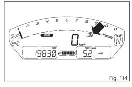
the low beam off: in this mode, the instrument panel automatically switches from the DRL light to the low beam and vice versa, according to the detected ambient light conditions. The display shows the green logo with letter A.
