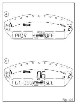
The list of devices found within the range during the Pairing stage does not include already paired devices, even if their Bluetooth connection is ON. The name of the device is scrolled on the display. To pass from one device to the other, press buttons (1) and (2).
