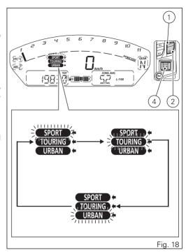
When system requests rider to confirm the riding mode change, the procedure will output an error if:
