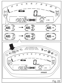
If the ABS is in fault, the instrument panel will display ABS lettering flashing, the dash "-" flashing and ABS warning light will be steady on.
