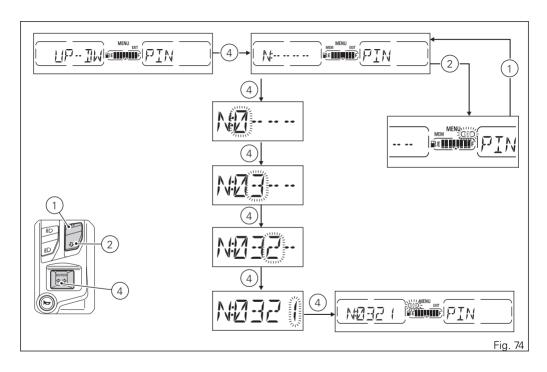
When you press button (4) to confirm the fourth and last digit, the instrument panel highlights the message "MEM" and the relevant box.
