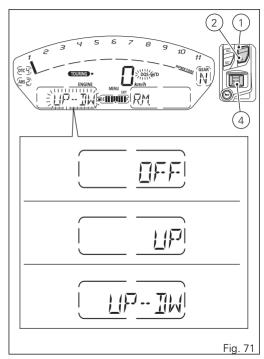
To exit the menu and go back to previous page, select "EXIT" and press button (4). The instrument panel will go back to the previous menu level and it will be possible to start the "Parameter storage" procedure.
