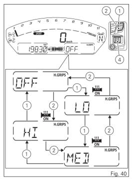
When the heated handgrips are ON, the relevant warning light turns on together with the indication "ON".
