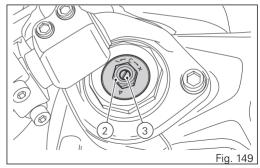
rebound: 3 turns (from fully closed); spring preload: 5 turns (from fully uncompressed).
