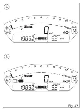
In case of missed calls from the moment the smartphone is connected to the bike to the moment it is disconnected, the missed call symbol will be displayed for one minute. The number of missed calls is not displayed.
