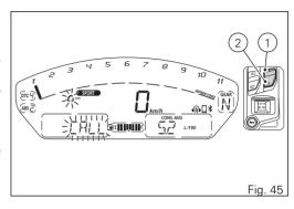
During the 5 seconds after hang-up, the Recall function is activated to allow the recall: Menu 1 shows the indication RECALL.
