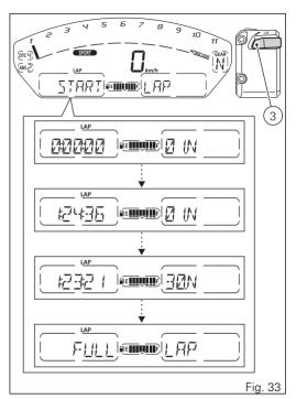
Laps are numbered from 01 to 30: after the first 30 laps, the instrument panel shows "FULL". If however the LAP function is switched on and the memory has not been cleared, but fewer than 30 laps have been saved (e.g. 12 recorded laps) the instrument panel records any left lap until memory is full (in this case, max. 18 further laps can be recorded).
