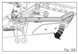
To ensure trouble-free operation of the side stand joint, thoroughly clean it and then use SHELL Alvania R3 grease to lubricate all friction points.
