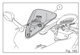
To move windscreen (1) from the low to the high position, grab it in the central area and pull it up, as shown in the figure, until hearing the "clicks" indicating the correct positioning of windscreen (1).
