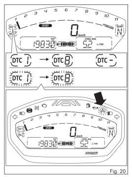
If DTC is in fault or the Black Box is in fault, the instrument panel will display DTC lettering flashing and "-" flashing and DTC warning light will be steady on.
