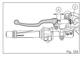
Adjuster (2), located on the lever, allows a maximum adjustment (Q) of 11 mm (0.4 in), whereas the standard adjustment (starting one) is of 5 mm (0.2 in). If working on such adjuster proves insufficient, work on the secondary adjuster (3).
